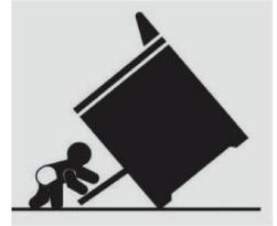
Do not operate the range without the anti-tip device in place and engaged. Failure to do so can result in death or serious burns to children or adults. Do not remove the leveling legs. Doing so will prevent the range from being secured by the anti-tip device.
