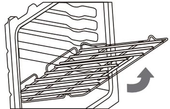
**Inserting Rack:** The rack can be installed in only one direction.
