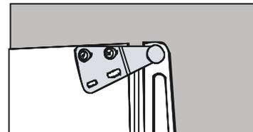
6) Slide the appliance door back on to the top hinge, making sure it's the right way up. Screw the bottom hinge into place on the new side. Replace the other foot on the other side. Replace the plastic covering by clicking back into position on the door hinge.
