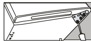
7) Check that the door is aligned horizontally and vertically and that the seals are closed on all sides before finally tightening the bottom hinge. Re-adjust the levelling feet.
