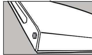
5) Remove the two screws from top bracket and replace on the other side. You will need to first remove the plastic caps from the other side.
