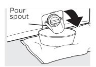
4. Turn the pump filter counterclockwise and remove the filter. Open slowly to allow the water to drain.
