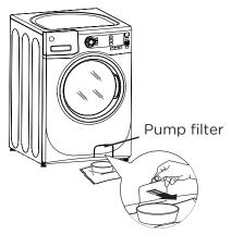
Using a coin or flat screwdriver in the notch on the door, open the access door.
