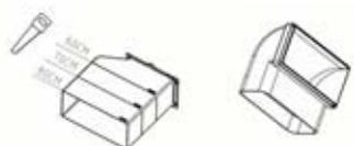
①—Pipe connector suitable for cabinets of different widths
