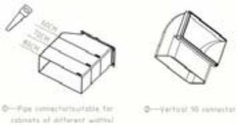
①—Pipe connector suitable for cabinets of different widths
