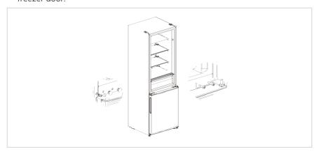
4. Dismantle the bottom hinge, hole caps and screws, Install the bottom hinge shaft on other side of the bottom hinge, then install the hinge on the other side.
