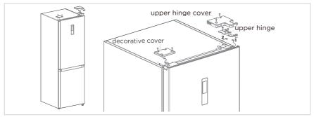
3. Remove the refrigerated door body (be careful not to lose small parts such as the shaft sleeve and stop on the door); Remove the middle hinge and remove the decorative cover of hinge hole on the other side.
