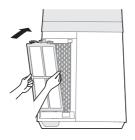
6 Install the air inlet grille: align the upper two buckles and press them tightly, then press the two sides at lower part, slowly and gently buckle the air inlet grille.
