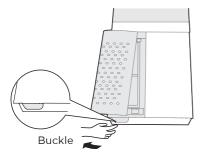
2 Take out the pre-filter: press the raised part on both sides to pull it outwards, and take out the pre-filter.
